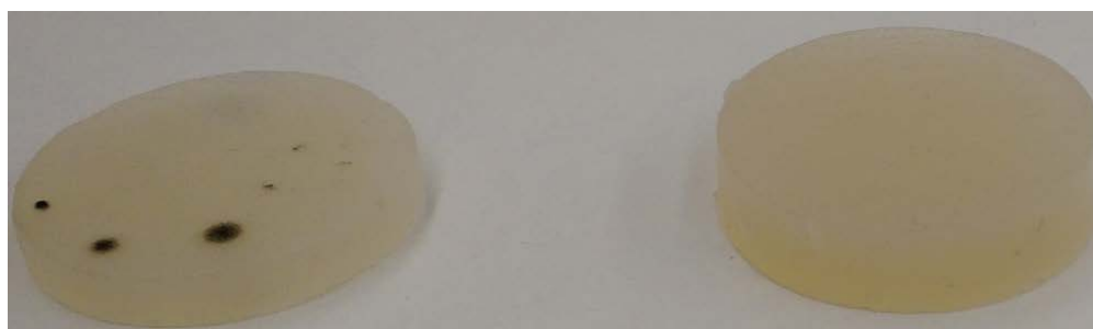
Figure 19: The sample on the left was untreated and mold growth is visible. The sample on the right was treated and no mold growth is visible.
