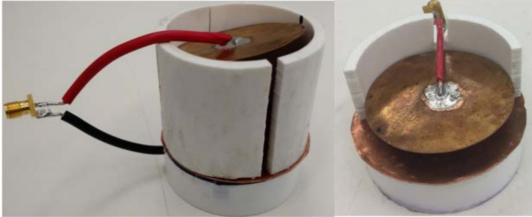
Figure 22: The network analyzer test fixtures are shown above. The fixture on the left introduced error in the measurements due to the long wires. The fixture on the right has shorter wires which led to more accurate data.
