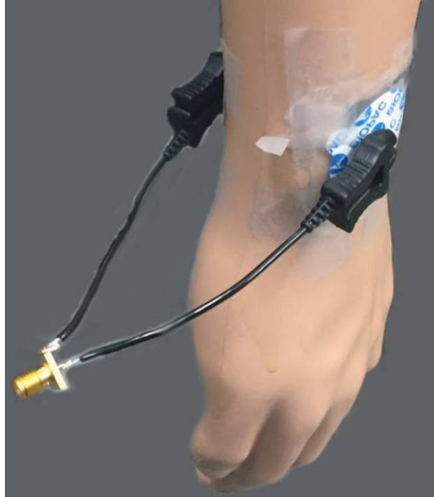
Figure 24: The phantom network analyzer test fixture is shown above. Identical test fixtures were used for each wrist to get the two port parameters.
